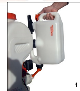
Fill up the tank by holding the can in vertical position (1). Sweep the can to empty the spout completely (2).
